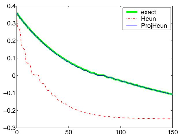
Figure 4.5: Rate of dissipation of the Heun and projected Heun method for the Duffing equation. Step size  $h = 0.5$ , starting value  $(1.6, 0)$  and time  $=[0, 150]$ .
