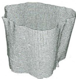
Fig. 11. Geometrical imperfections for cylinder AL-1100, scaled by factor of 50.
